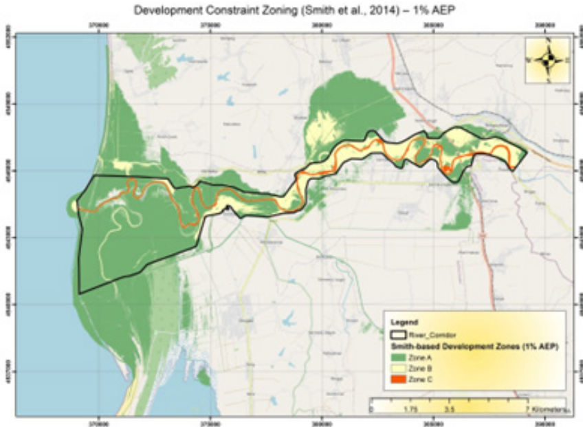
Figure 9: Flood hazard zoning map according to Smith et al. (2014) for the 1% AEP event
