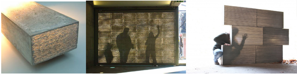
Figure 1 LiTraCon blocks (Light Transmitting Concrete blocks)
