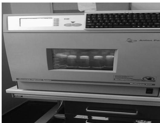
Photo no. 2: Microwave device which enables the nitric acid to warm up in the tubes and allows the organic matter present in the soil and other elements to enter the nitric acid solution and then read by IPC-MS.
